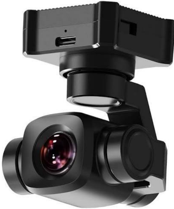
Figure 1. SIYI A8 mini gimbal camera: 95 g, 3-axis stabilized, 1/1.7 in Sony sensor behind a fixed 21 mm equivalent lens. Ethernet output rather than optical performance is what decided the selection — it carries two independent video streams at once.
