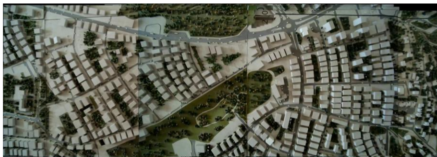
Figure 5. First stitching test, imagery captured over a scale model. No coordinate data is used — each frame is placed relative to its neighbor — and the upper and lower edges of the mosaic step rather than running straight.
