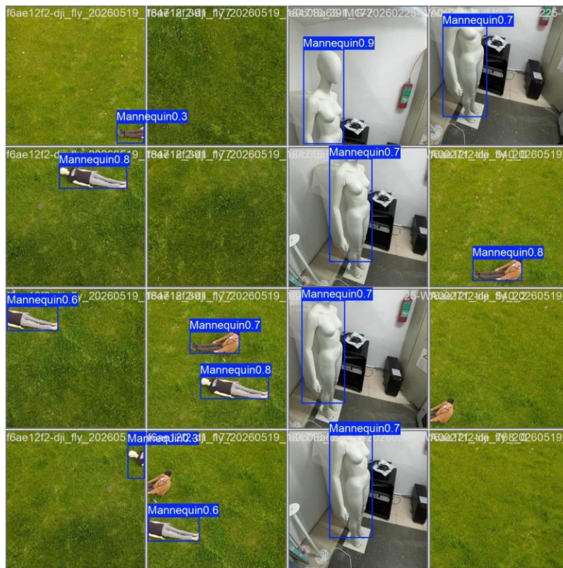
Figure 4. Validation predictions with confidence scores, aerial and studio mannequins mixed. The high-confidence boxes are fully exposed targets and the low-confidence ones are partially framed. Two miss cases are visible in the bottom-right tiles — a mannequin is present and no box is drawn.
