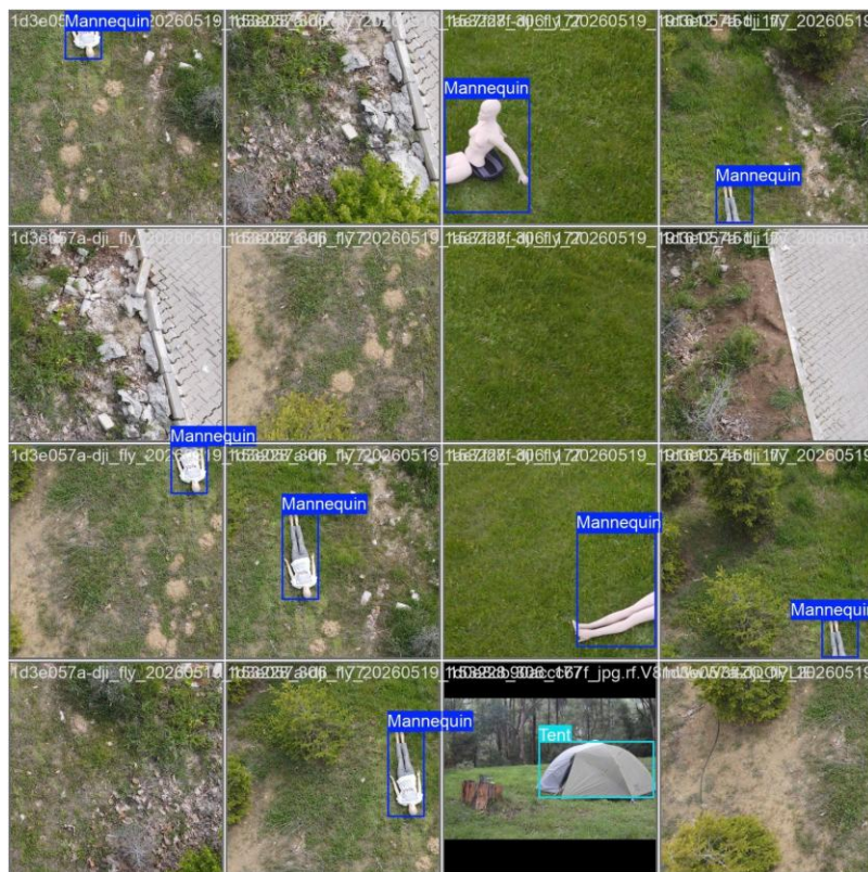
Figure 3. Labeled mannequin and tent instances in real drone imagery. Two things are deliberate and worth noticing: several tiles carry no box at all — frames of bare grass, gravel and paving are kept in the set as negatives — and several boxes enclose only a pair of legs, which are the partial-occlusion cases.
