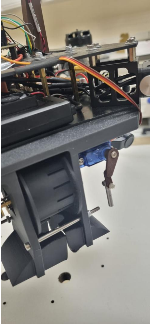
Figure 3. The assembled plate stack, photographed from the side. The spacers standing between the two plates are the load-bearing members described here, and the wiring runs through the gap they open. The photograph also shows a servo and a mechanism below the lower plate that this document does not describe.
