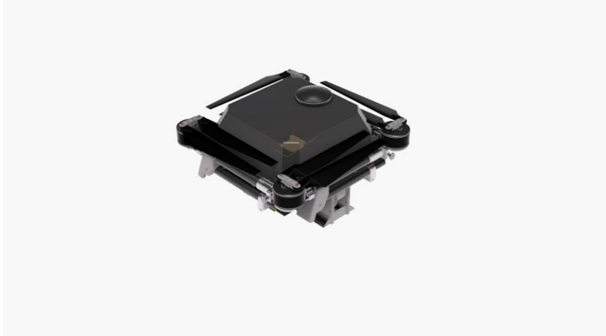
Figure 5. The aircraft folded for transport, from the CAD model. The arms have swung back alongside the body and the legs have collapsed against it; this is the 13 x 13 inch configuration referred to in the text.
