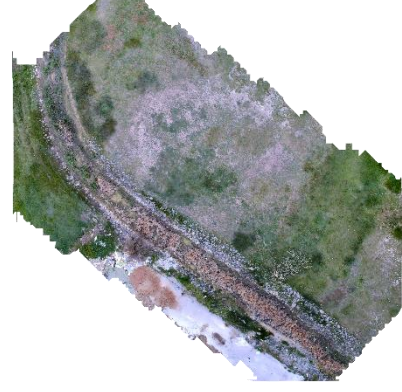
Fig. 1. Stitched map produced by the FastMosaic pipeline from survey imagery collected during a waypoint tour.
