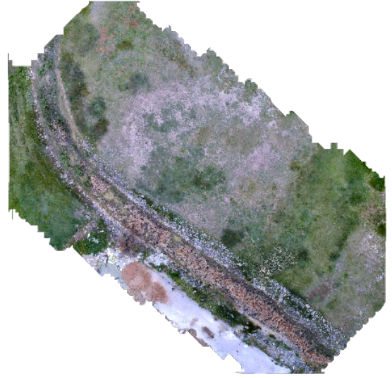
Fig. 7. Stitched map produced by the FastMosaic pipeline from survey imagery collected during a waypoint tour.
