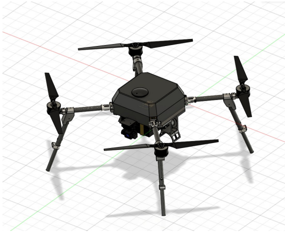
Fig. 1. CAD model of the UAV airframe showing the carbon-fiber arms, foldable joints, main plates, and the folding landing gear in the deployed configuration.
