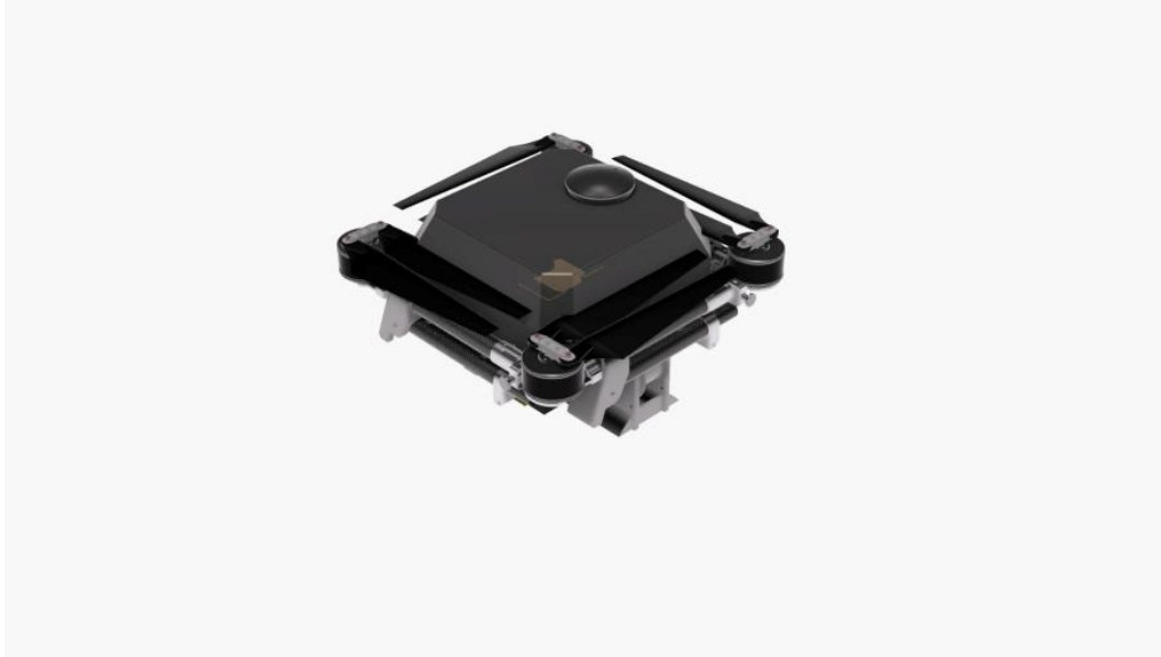
Figure 9. The aircraft folded for transport. The carbon-fiber arms and telescopic landing gear are retracted to produce the 13 x 13 x 7.1 inch transport configuration.
