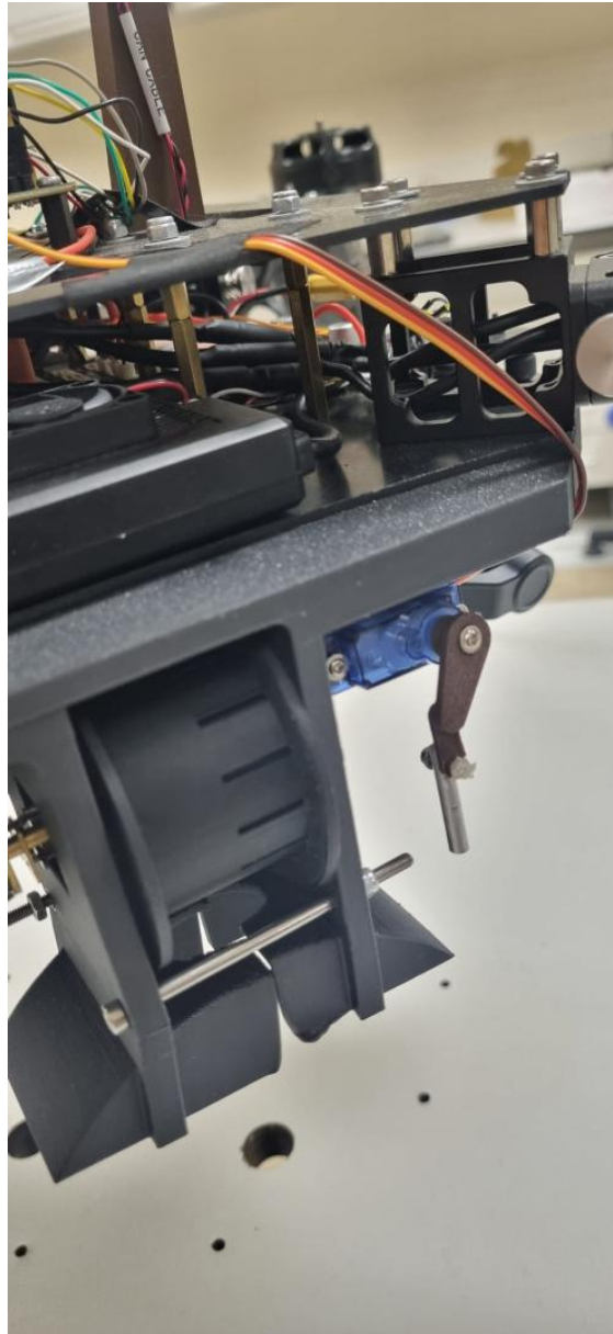
Figure 3. The assembled plate stack. The spacers connect the main plates and create an internal volume for wiring and subsystem installation.
