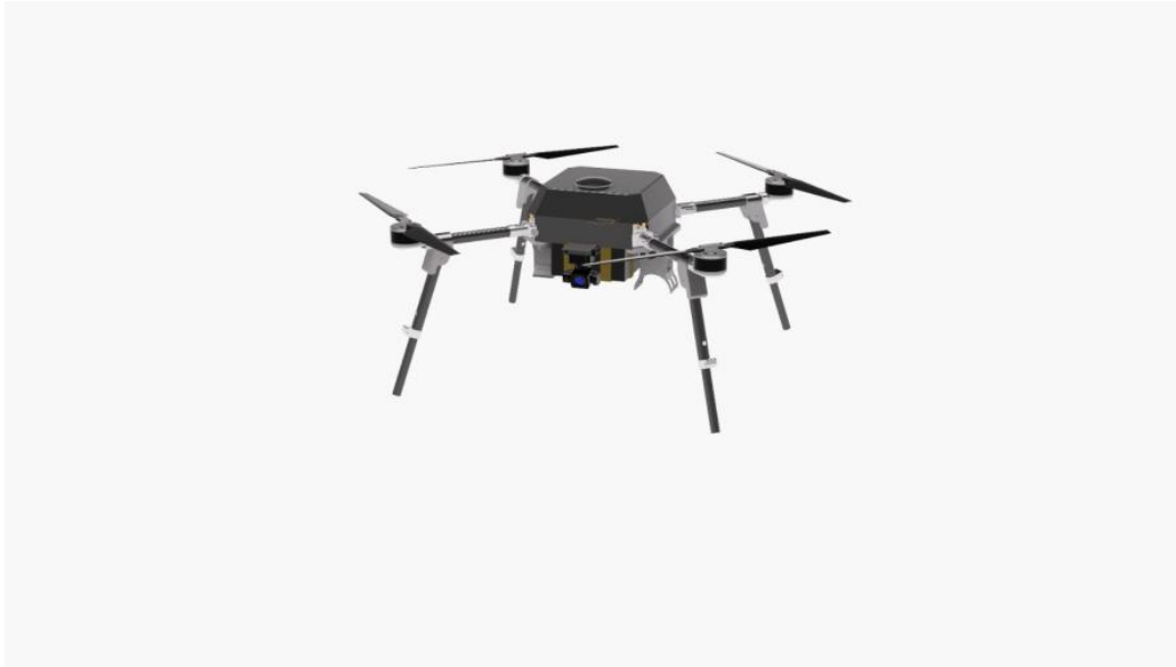
Figure 1. The airframe in its deployed flight configuration, from the CAD model. The carbon-fiber arms and telescopic landing gear are fully extended for flight.
